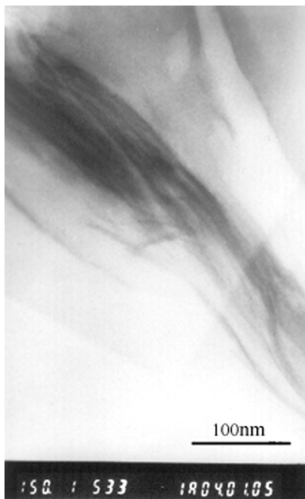
Figure 3 TEM image of PET/HTPP-MMT nanocomposite with 3 wt % MMT loading.
